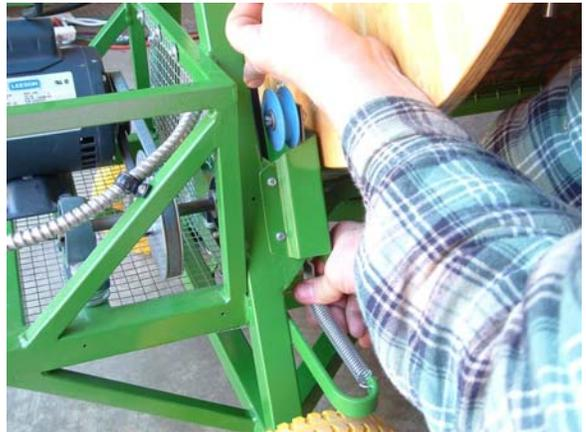
After releasing the belt and the tension arm, the belt should be positioned outside the idler pulley as in the photo to the right.
