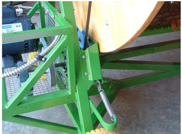
Step 2: Reach a little farther into the tumbler frame and pull the lower end of the other tension arm toward yourself until you can lift the belt and slip it forward toward the open end of the shaft. After releasing the belt and tension arm, the belt should be relaxed, and resting outside the idler pulleys.
