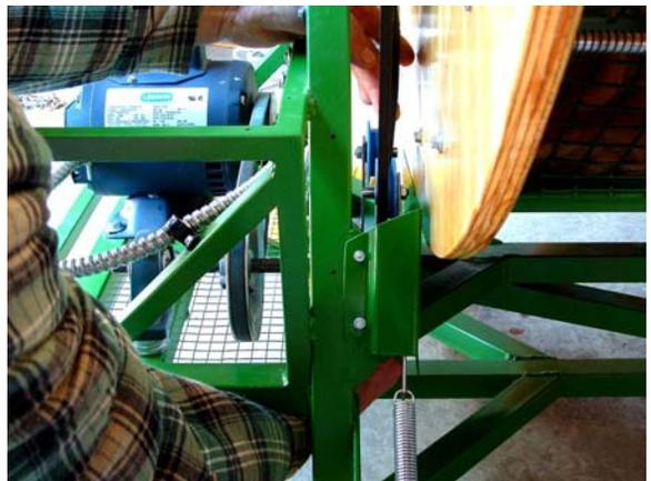
Step 3: The belt can now be slipped off the large upper pulley and the lower drive pulley, and then threaded upward past the idler pulleys.
