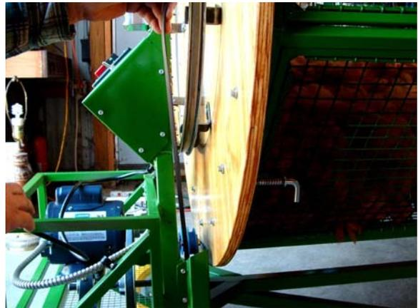
Step 4: **Caution:** Because the tumbler cage is very heavy, it would be advisable to remove all 6 panels from the cage to reduce weight. The tumbler must be placed on a level surface so the pillow-block bearing does not slide off the frame after the carriage bolts are removed.
