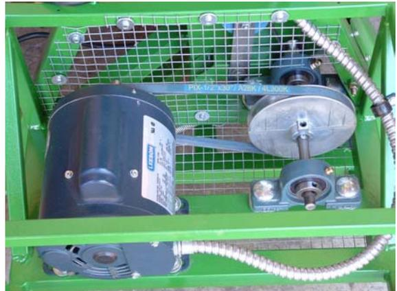
**Step 5:** The V-belt can now be slipped off the pulleys and removed.
