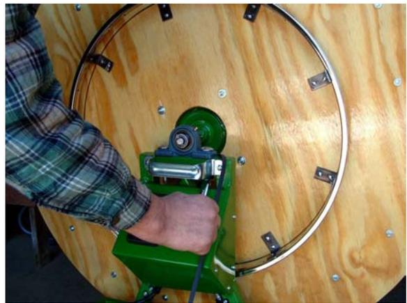
Step 5: **Caution again:** You must make sure the pillow-block bearing remains directly above the frame surface when lifting it so that it will fall onto the frame if it slips from your grasp. It may be advisable to have a second person remove the belt while the first person raises the pillow-block bearing slightly.
