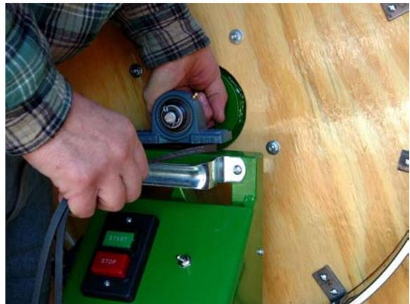
Step 6: Installation of the new belt can be accomplished by following steps 1-5 in reverse order. Be sure to install the belt with the ribbed side **facing** both the drive pulley and the large pulley. The back side of the belt should be facing the idler pulleys. And, be sure that the belt correctly engages the ribs in the lower drive pulley. Also, double check to make sure there are no twists in the belt. When finished, the belt should be arranged as shown in the photo to the right.
